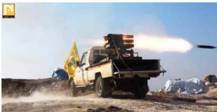
107mm rocket being launched from a multi-barrel launcher carried on an off-road vehicle (Nujaba Movement's Twitter account, June 11, 2022)
