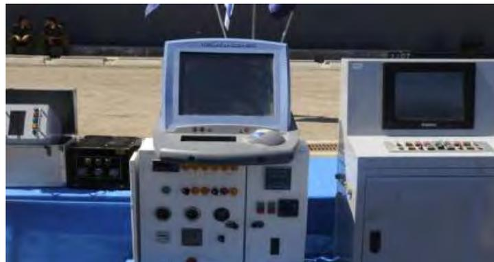
Radar monitoring and control stations on board the ship (IDF Spokesman, March 16, 2011).
