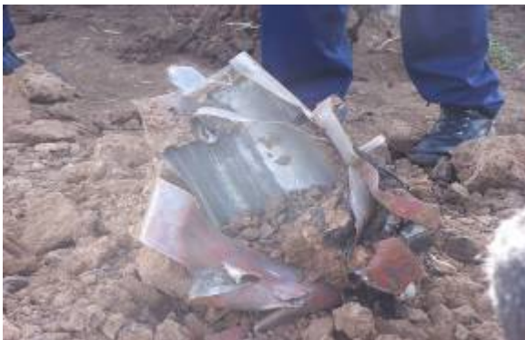
Part of the tail of a Chinese 122mm rocket, maximum range, 40 km.
