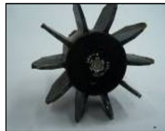
120mm mortar shell tail fired during the second Lebanon war
