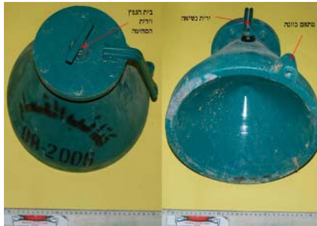
Hamas's homemade Shawaz ("flame" in Arabic) EFPs. They have higher penetrating capabilities than the IEDs usually used by the Palestinian terrorist organizations (estimated at more than 200mm of steel).
