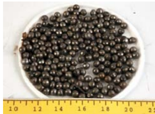
Ball bearings in the warhead of a Chinese 122mm rocket to kill and maim civilians – range, 40 km.
