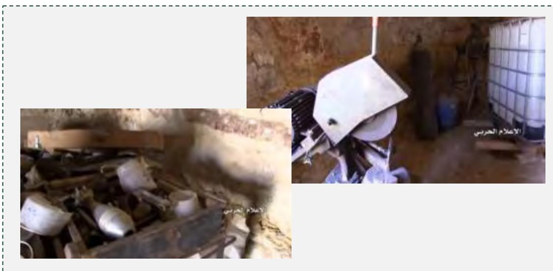
Weapons and equipment found in the workshop. Right: Bench grinder and an oxygen cylinder (for welding) that were used to manufacture mortar shells and rockets. Left: Mortar shells manufactured in the workshop (Hezbollah’s Military Spokesman’s Office, July 28, 2017).
