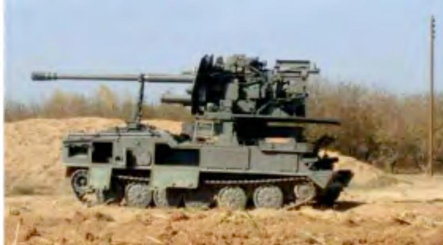
100 mm self-propelled anti-aircraft gun on a hull for an SA-6 anti-aircraft missile system (As-Safir, November 16, 2016)
