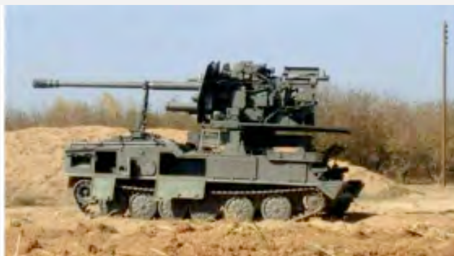
100 mm self-propelled anti-aircraft gun mounted on a hull for an SA-6 anti-aircraft missile system (As-Safir, November 16, 2016)
