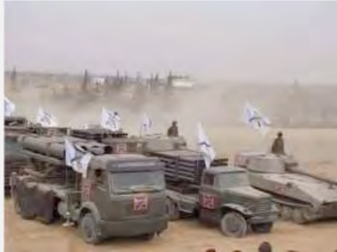
The truck on the left carries a 302 mm rocket launcher (estimated range of 90-180 km). The first truck in the middle carries a 122 mm rocket launcher. On the right: a 122 mm self-propelled gun (Al-Hadath News, November 22, 2016)
