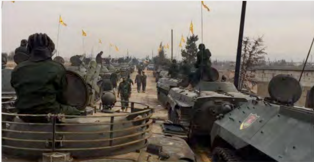
A column of Hezbollah's armored vehicles, including APCs, tanks, and self-propelled guns, which appeared in the military show of strength held in the Syrian city of Al-Qusayr (Araby 21, November 14, 2016). Right: The second and third APCs were identified as BMP of Soviet origin. Left: APC identified as BMP-1, with a Sagger anti-tank missile on it.
